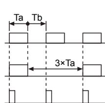
Ta(ON width) and Tb(OFF width) need to be over min. signal width.
