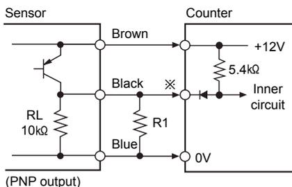
※Please set R1 value to make the composed resistance of  $RL + R1$  as Max. 470kΩ is an impedance for short-circuit.
