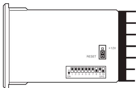
※ Inner selection switch is changed from 8pin to 10pin with upgrade of counting speed.
