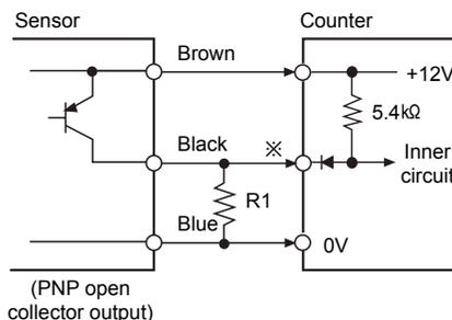
※In case of PNP open collector output type sensor, please connect lower than 470Ω of R1 to input terminal before using.
