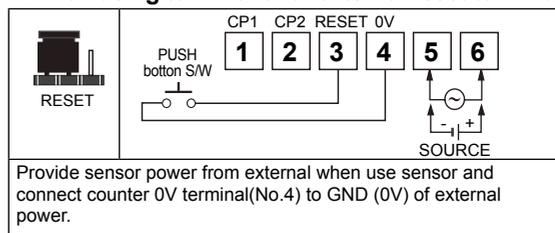
Provide sensor power from external when use sensor and connect counter 0V terminal(No.4) to GND (0V) of external power.
