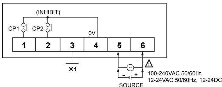
※1: It can be selected RESET or sensor power(+12VDC 50mA) by internal PIN operation.(Refer to J-40)
