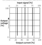
It outputs a constant current proportional to the control input so that the output current does not fluctuate against fluctuations in power voltage and load resistance fluctuations of loads (platinum, molybdenum, tungsten, etc.) in which the temperature coefficient of electrical resistance varies significantly from 6 to 12 times the normal
