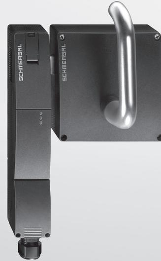
Solenoid locking switches are used on sliding, hinged and removable guard doors that must be closed and locked for operator safety. It is a two part system consisting of a switch body, mounted to the guard frame, and a separate actuator key, mounted to the door.
