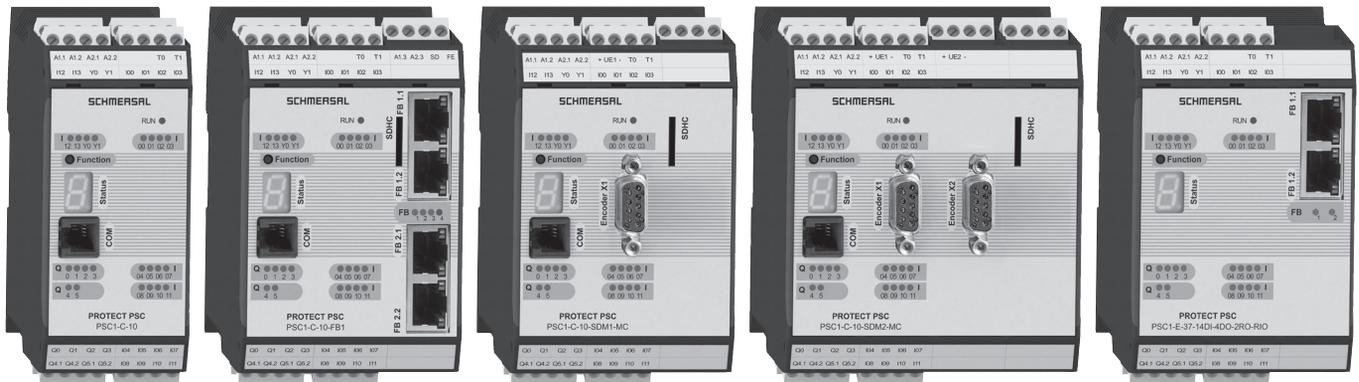
The safety control system PSC1 consists of freely programmable compact safety controllers with I/O extension modules for signal processing of emergency stop switches, guard door switches, light grids and additional mechanical and electronic safety switchgear. Additionally there is the possibility via numerous functions to monitor axes. Using the universal communications interface, a connection can be established to all standard field bus systems.
