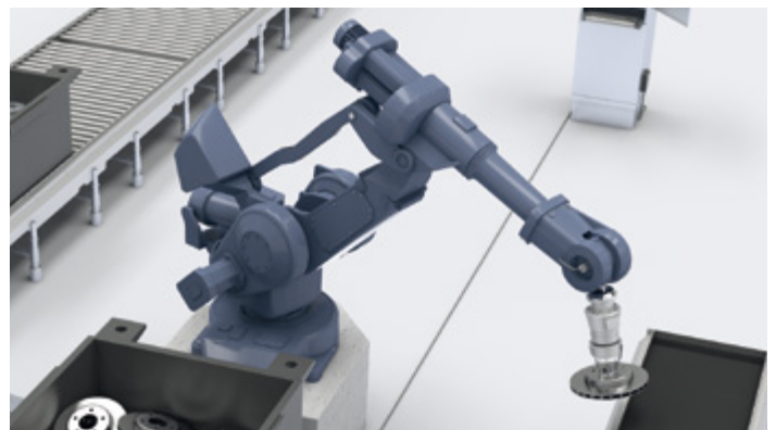
The small magnetic rotary encoder controls the rotation of the robot arm and ensures reliability in the production process.
