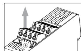
Lift the lower part of the terminal unit  $\uparrow$  upwards by using a tool (e.g. flat-head driver).
