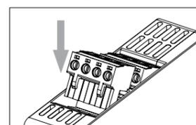
Press the terminal unit downwards to insert.
