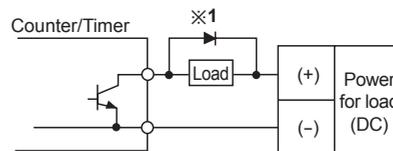
※For solid state output, select load power and load not to be over (max. 30VDC, 100mA), switching capacity.
