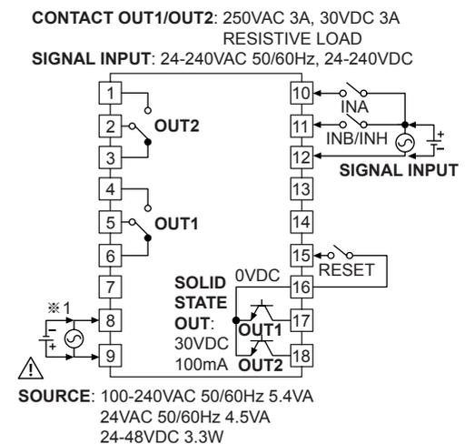
※1: AC voltage type: 100-240VAC 50/60Hz
