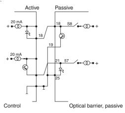
S7: ON = input interface active, 20 mA current loop
