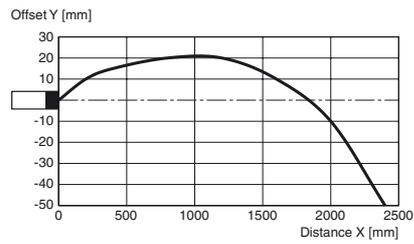
Permissible distance (offset) between optical axis and object.
