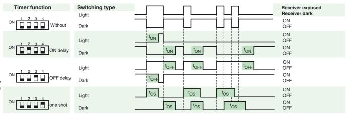
Time  $t_{ON}$ ,  $t_{OFF}$  and  $t_{OS}$  are adjustable from 0.02 to 1 seconds.
