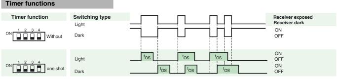
The Light-/Dark-Switch (Left, outer switch) is shown in the "Dark ON" position.
