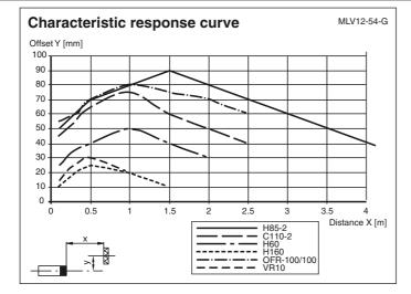
Retroreflective sensor with polarization filter for clear object
