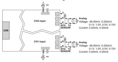
$\ensuremath{\mathbb{X}}$  Input parts and USB cable connection part are insulated each other.
