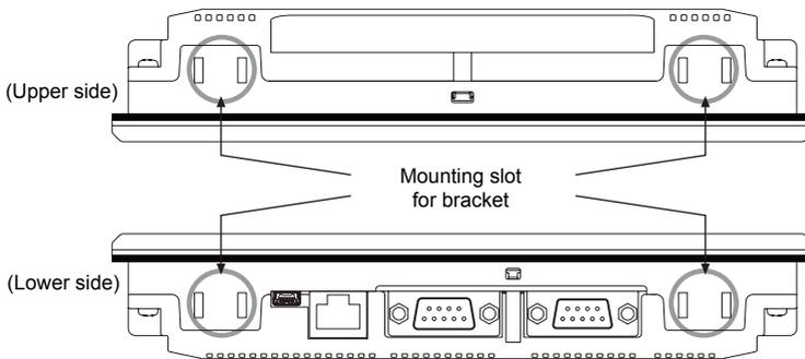
3. Tighten fixing bracket with M4 Screw driver and tightening torque is 0.3 to 0.5N·m.
