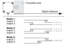
A1  $\rightarrow \infty$ , A2  $\rightarrow \infty$ : Object presence detection. Both outputs operate according to the selected mode, if an object is located within the detection range.
