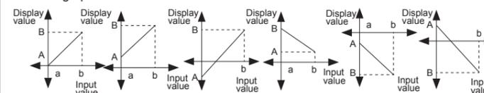
Display scale function is able to change display value for max./min. measured input by setting high limit scale [H-5C] and low limit scale [L-5C] in program mode.
