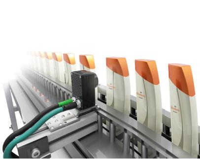
Sensing presence or defect of the syringe rubber seal
