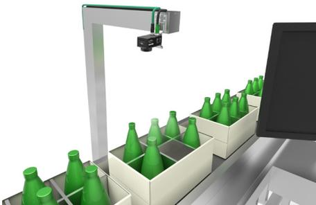
Sensing the printing and marking status of the package
