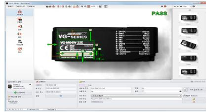
※Vision sensor is connected with Vision Master in Ethernet (TCP/IP) communication.
