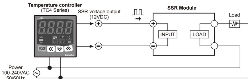
※When selecting phase or cycle control mode, the power supply for load and temperature controller must be the same.
