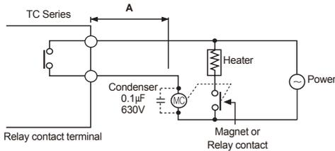
Keep **A** length as long as possible when wiring the temperature controller and the load. If wire length of **A** is short, counter electromotive force which occurs from a coil of magnet switch & power relay may flow in power line of the unit, and it may cause malfunction.
