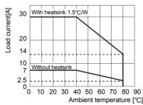
♠Please supply less than 50% of the rated load current when installing several SSRs closely due to decreasing effectiveness of protection against heat.
