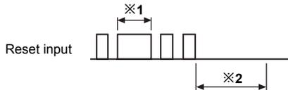
※1: In case of a contact reset, it is reset perfectly if the ON time of reset signal is applied during min. 20ms even though a chattering is occurred.
