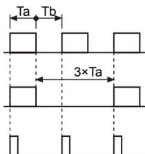
$T_a$ (ON width) and  $T_b$ (OFF width) need to be over min. signal width.
