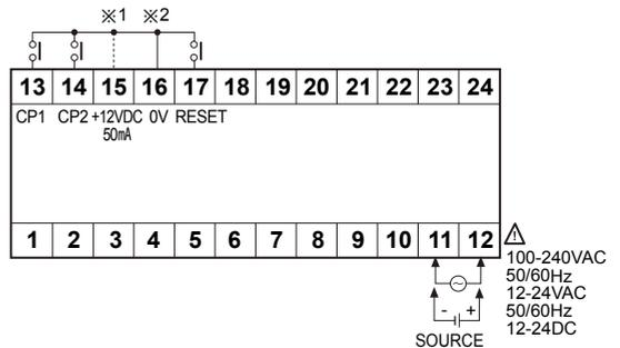
※1: Connection for PNP input in contact input
